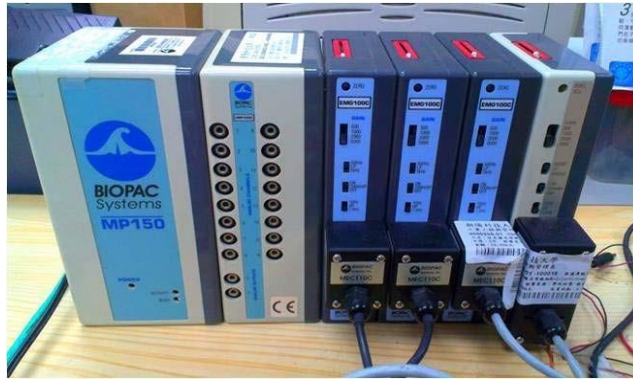
Figure 4. Biopac MP150 myoelectric signals measurement recording system
